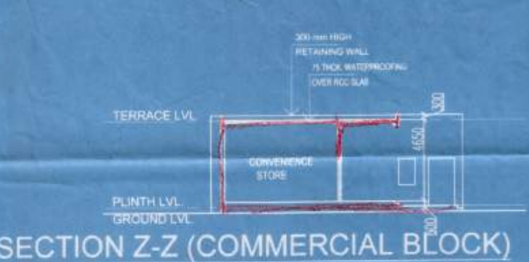
SECTION Z'-Z' (COMMERCIAL BLOCK)
